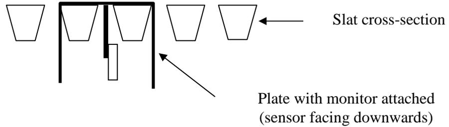
**Figure 7** Typical installation of monitors within the slat system
