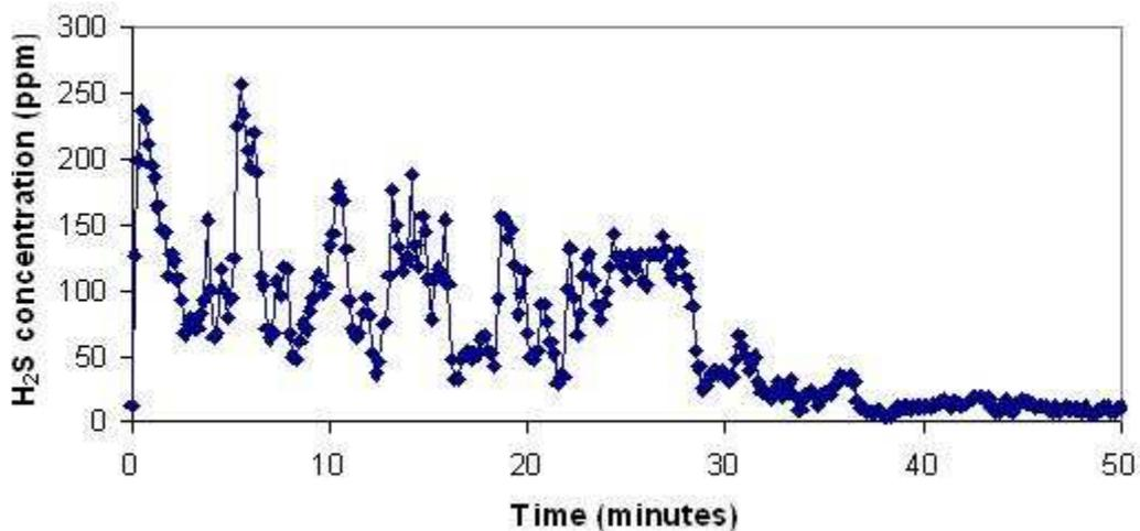
**Figure 10** Concentration of H<sub>2</sub>S detected during mixing of non-aerated slurry in tank 1 at slat invert level.
