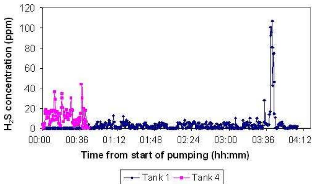
**Figure 11** H<sub>2</sub>S concentrations recorded 0.5m above centre of tank 1 and at slat invert level for tank 4 during pumping of non-aerated mixed slurry
