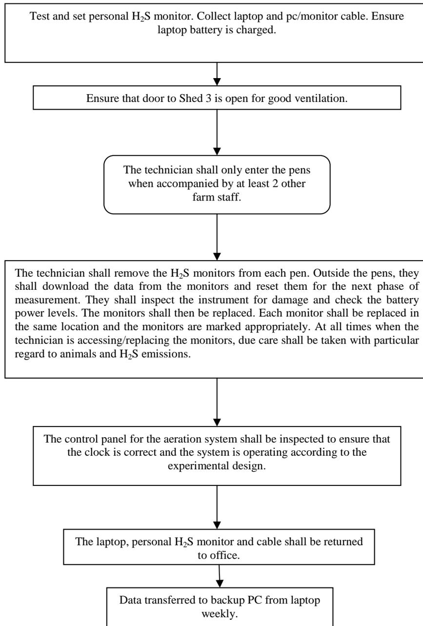
**Figure 3 Protocol for weekly collection of H<sub>2</sub>S data from monitors**
