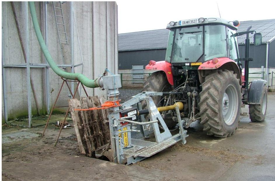
**Figure 8** Slurry pumping from reception pit to above ground tank
