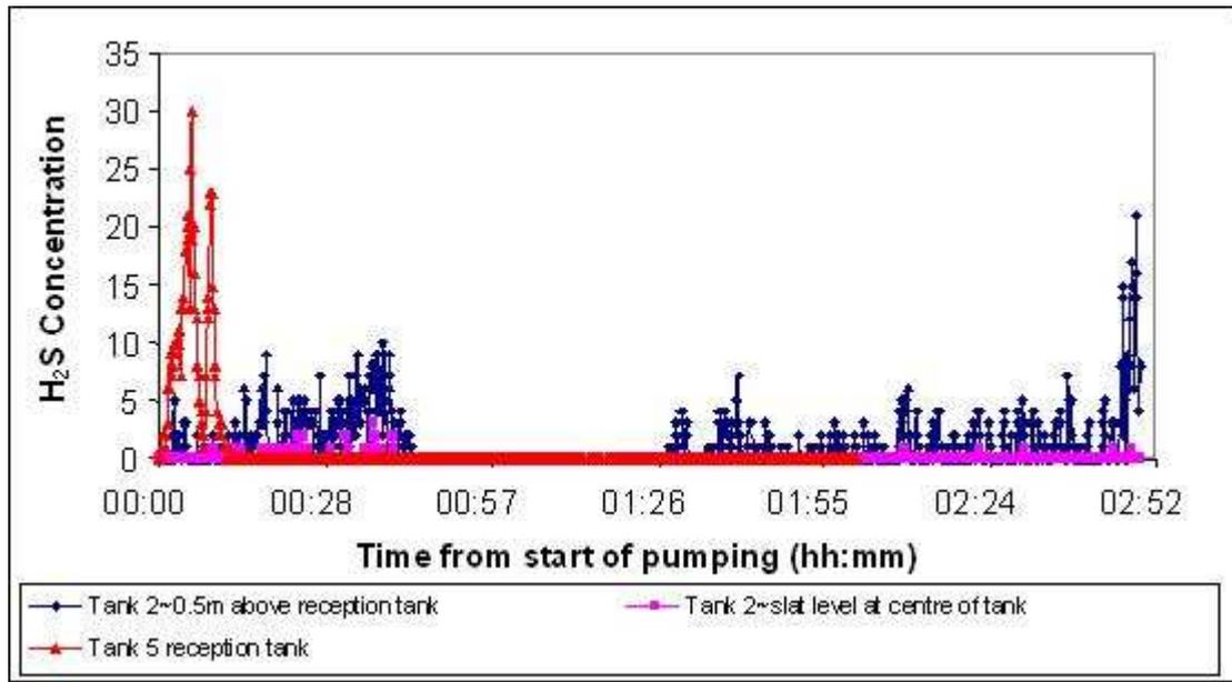
**Figure 9** Concentration of H<sub>2</sub>S detected during pumping of aerated slurry at slat level for tank 2, above the pumping point for tank 2 and at slat level of reception tank for slurry being pumped from tank 5.
