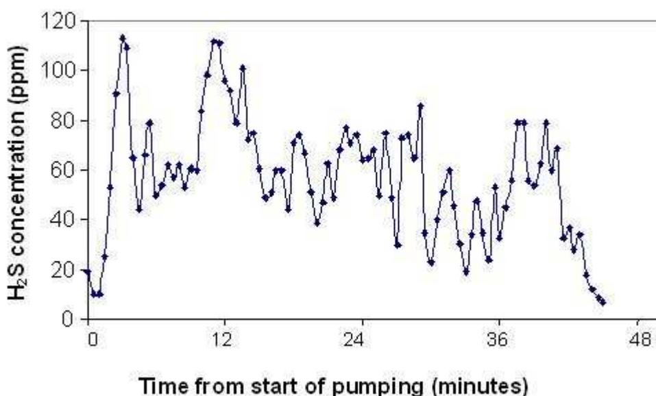
Figure 12 H<sub>2</sub>S concentrations recorded in centre of reception tank beneath slat level during pumping of non-aerated mixed slurry from tank 4.
