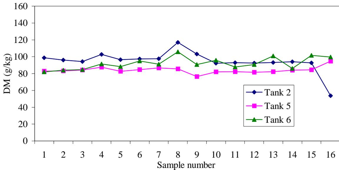
**Figure 15** Dry matter of slurry samples taken from aerated slurry tanks at various depths after animal housing period
